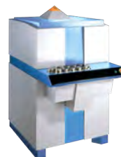
ARL 9900 X-ray WorkStation full XRF/XRD
