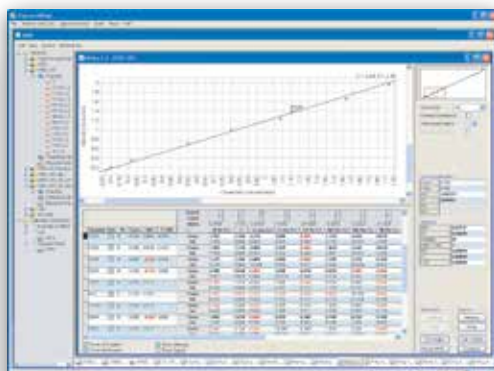
MVR calibration curve: real concentrations vs. intensities
